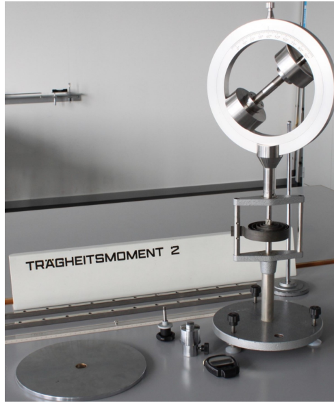
Figure 1: Setup used in the experiment. For the first two parts, the dumbbell was replaced with two beams (and a disc) (source: [1])
